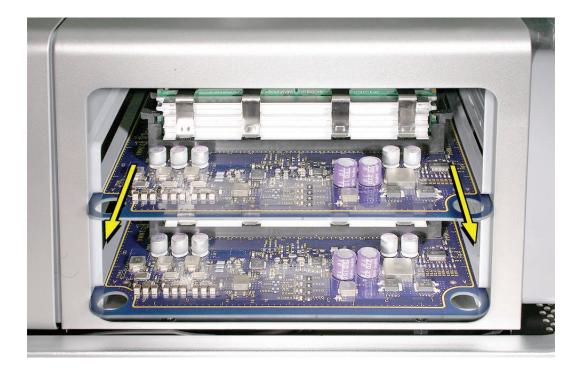
4. Open the ejectors on the DIMM slot by pushing them out to the sides, and remove the FB-DIMM from the riser card.
