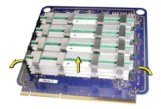
Warning: FB-DIMMs carry heatsinks on either side of the DIMM. Never attempt to remove the heatsinks from the DIMMs. Doing so could damage the DIMM.
